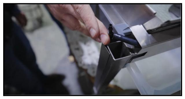
(Image shows T-connector lined up to leg. Extra metal clip is the WATERLINE ENCLOSURE leg cover which will be attached once the rack is completely assembled and only if this add-on was purchased with your rack.)
