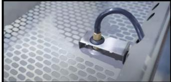
20. ONLY IF YOU ORDERED WATERLINE ENCLOSURES WITH YOUR RACK: Place valve covers over valve location (there is a small piece on the back of each cover that will need to be slightly bent down - can be done by hand) and be sure small tab is slotted into the back of the valve clip. Press down until the cover clips into place. See images below.
