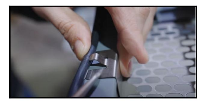
13. ONLY IF YOU ORDERED WATERLINE ENCLOSURES WITH YOUR RACK: Slide valve sections of water lines through each corresponding slot on the back of the waterline enclosure and clip (back-side first) over the top of the waterline. Be careful not to pinch the waterline while pressing down. See image below.
