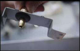
19. Attach the waterline ends to the valve and slide edge under the front of the rack frame. Press in until (two dimples) pop into place. Valve should perfectly line up with the valve hole on insert. See image below.
