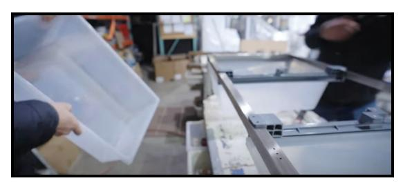
(Add tubs to channels BEFORE riveting to ensure even fit.)
