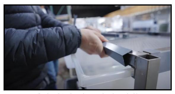
(Attach ventilation clips to the front of the rack for each tub.)
